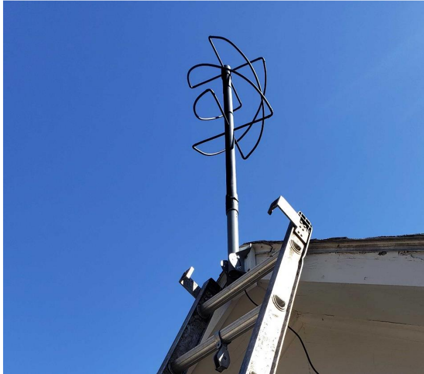
My completed Antenna Note: the mount I used is called a roof/deck mount, new, costs about $13.99 My whole antenna build was about $29 plus the mount. The mount is conveniently 1 ¼" and matches the PVC exactly.
